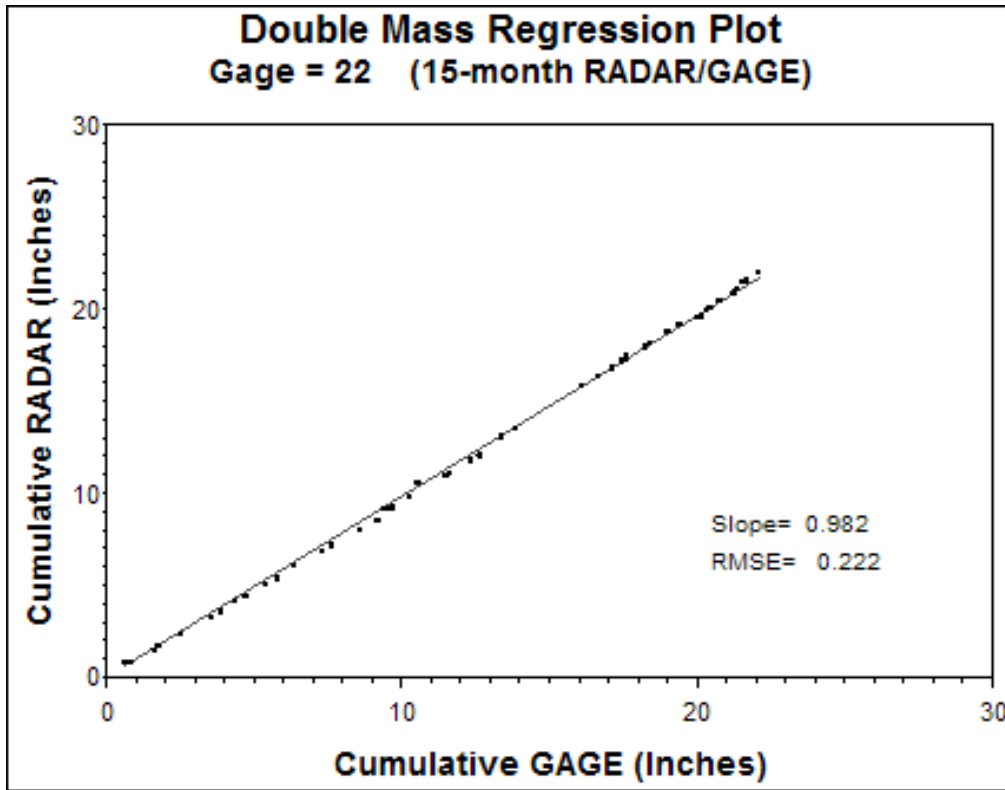
Figure v5-23 Double Mass Regression Plot of Cumulative Daily Radar Against Gage Rainfall Totals at PWD Rain Gage 22 for the 15-Month Radar Study Period
